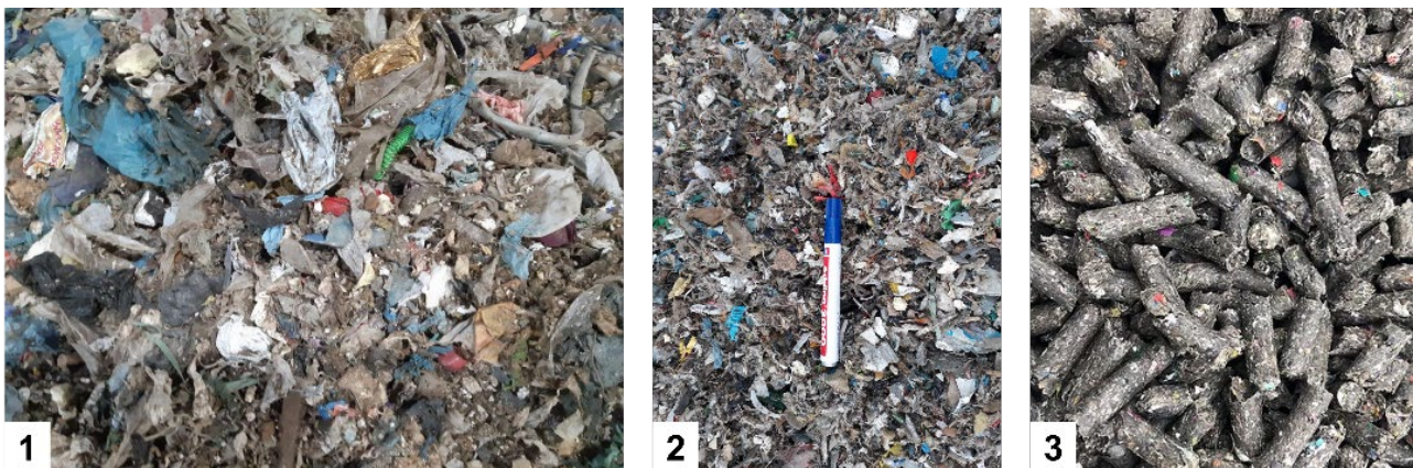
Figure 8: Various RDF qualities, 1) medium quality SRF acc. to Sarc [11], 2) premium quality SRF acc. to Sarc [11], 3) pelletized RDF [19, 20]
