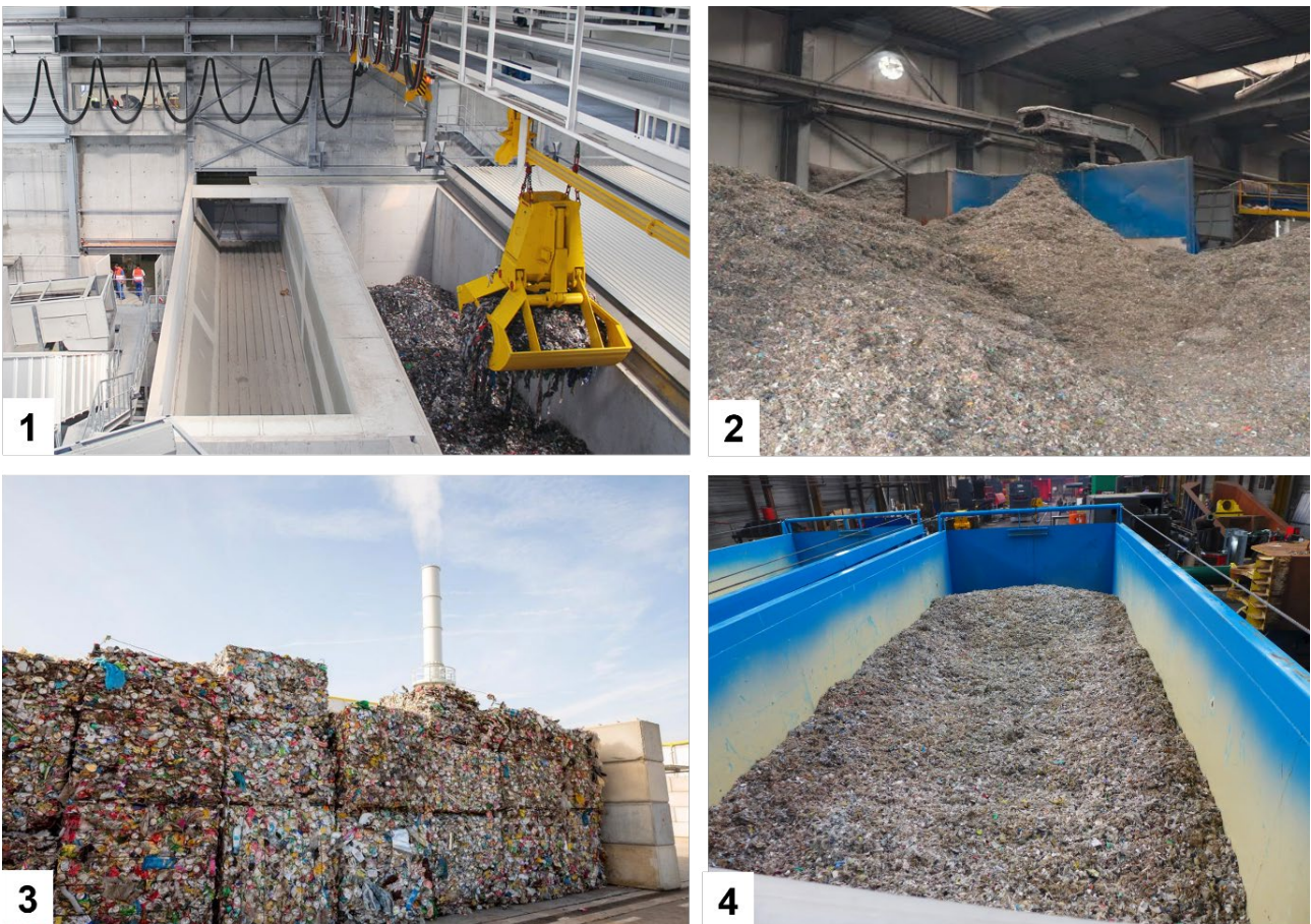
Figure 15: Various storage types of RDF, 1) deep bunker acc. to [43], 2) alternative fuel storage at the production and storage hall acc. to [44], 3) bale stack acc. to [45], 4) storage box acc. to [46]
