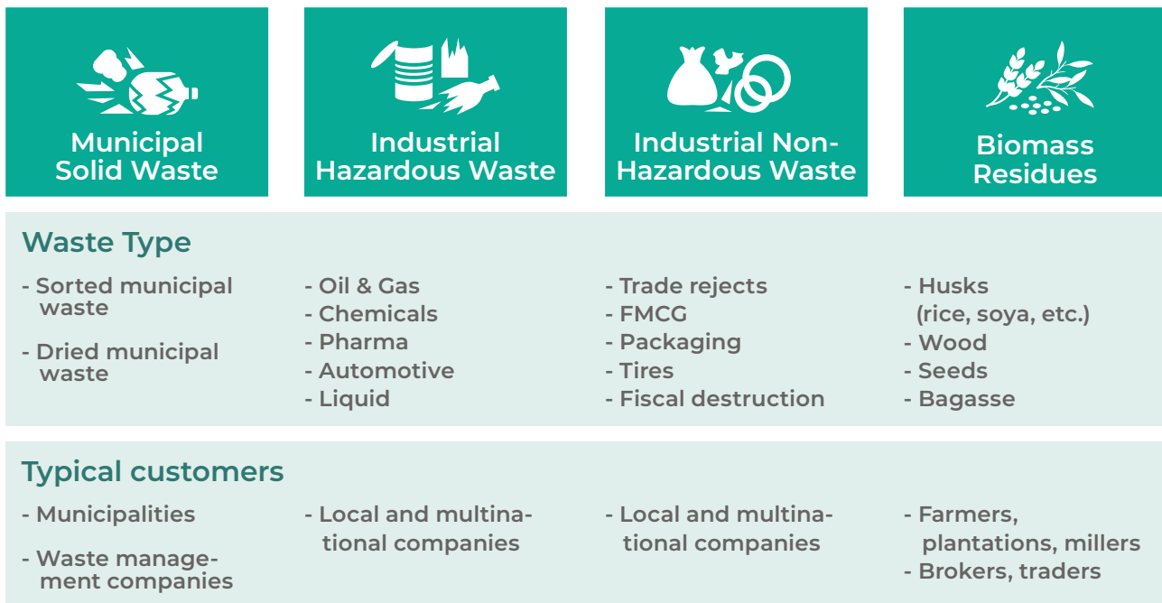
Figure 6: Waste types relevant for pre- and co-processing in the cement industry [13] (modified)
